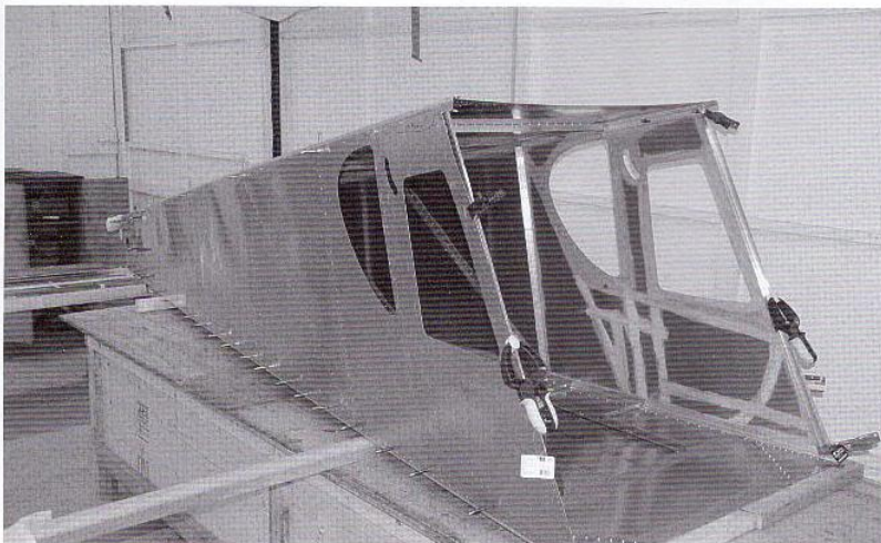
The Cruiser goes together quickly. The kit chosen was not a quick build since part of the rationale was to maximize participants learning opportunity. The aft fuselage is shown here: a way to go, but it's starting to look like an airplane.
