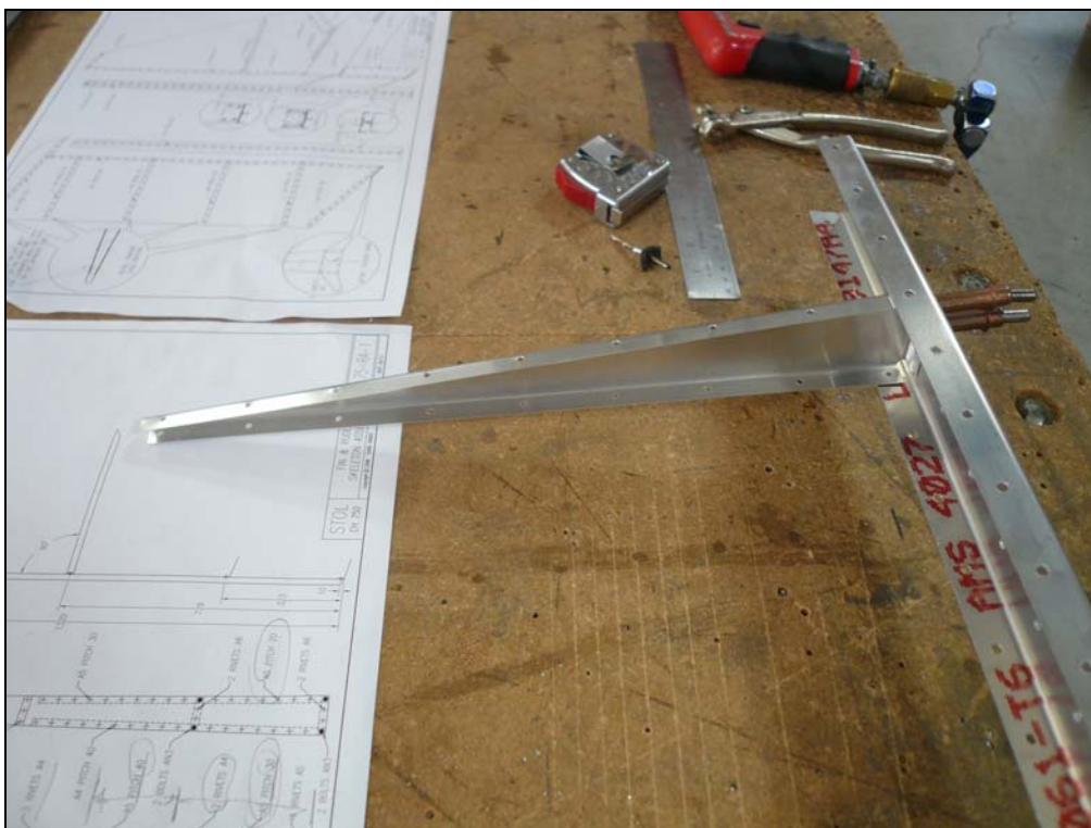
P/N: C75R1-5 Rudder Rib #4
